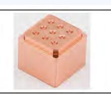
Typical Point: 1. The sample processed accurately, the error between the center of each hole is within ±0.002 mm. the maximum diameter error of the 29°taper flat surface is controlled in ±0.005 mm.
